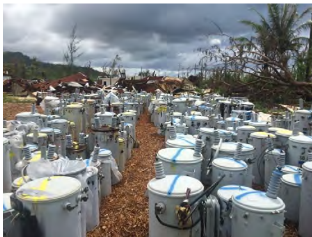
Figure 26. Waste caused by Typhoon Soudelor included 733 transformer carcasses and six drums of transformer oil contaminated with polychlorinated biphenyls, or PCBs.
